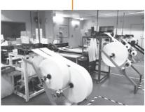
**Cutting** of the raw material into wipes (cleanroom ISO 6)
